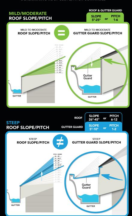
You will need to use one of the bending methods shown on p. 13 to achieve the recommended installation slope.
