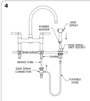
**Please note:** If there is a low flow at the hand spray, reinstall the side spray connector: Remove the hose and follow the instructions in step 3.
