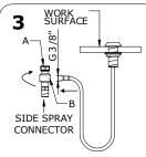
DO NOT INSTALL THE SIDE SPRAY CONNECTOR ONTO THE UNION AND THEN INSTALL THE HOSE.
