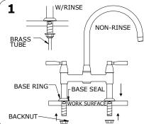
Ensure the mixer is orientated correctly, levers should rotate to point forward.
