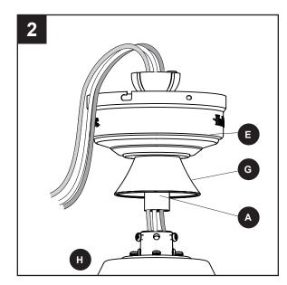
3. Slide the downrod (A) into the yoke, align the holes, then re-install the downrod pin (B) and downrod clip (C). Secure with set screws (I) and slide the yoke cover (G) down until it rests on top of the motor assembly (H).
