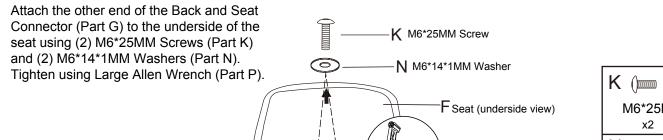
NOTE: Do not use the first set of holes in the extender portion of the Back and Seat connector. That will insert into the Control Mechanism in Step 3.
