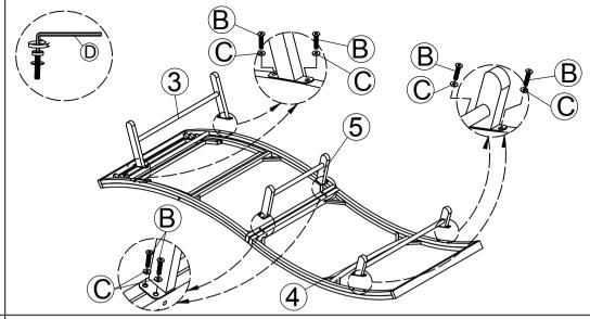
STEP 2: Connect Long Leg (3), Short Leg (4), Middle Leg (5) & The Part from Step 1, tighten Bolt (B) & Flat Washer (C) with Allen Key (D).
