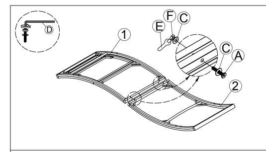
STEP 1: Connect First Frame (1) & First Frame (2), tighten Bolt (A), Flat Washer (C) and Eru (F) with Allen Key (D) and Key (E).
