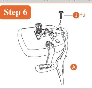
Align the screw holes of the Backrest (A) and Mechanism (D). Using Wrench (Q), secure both completely with Bolts (J)\*3.
