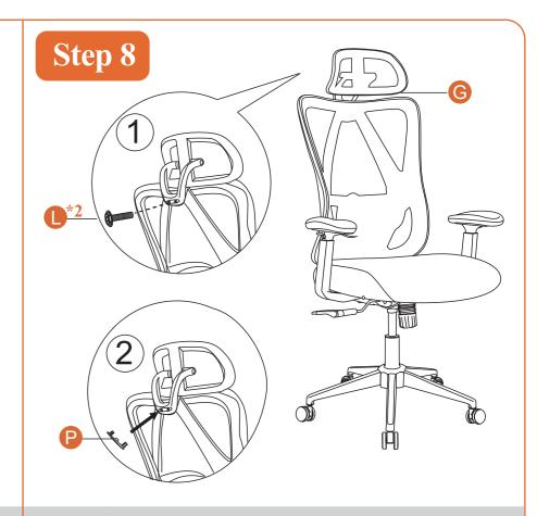
Using Wrench (Q), attach Head Pillow (G) to the Backrest (A) with Bolts (L)\*2. Then, attach the Plastic Cover (P) to the hole.
