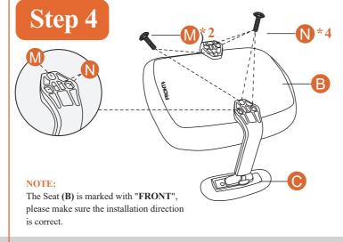
Turn the Seat Cushion(B) upside down. Install Armrests (C)\*1L\*1R to the Seat (B) with Bolts (M)\*2 and (N)\*4.
