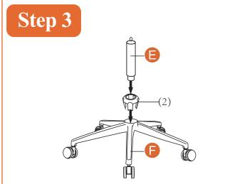
Put Base Cover (2) back on the Base. Then insert Gas Lift (E) into the center hole of the Base (F).
