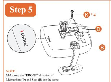
Attach Mechanism (D) to the Seat Cushion (B) with Bolts (K)\*4.
