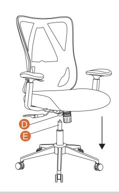
Align the hole on Mechanism **(D)** with Gas Lift **(E)**, and press the Chair down until it is fully secured.
