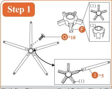
Divide Base (F) into two parts, (1) and (2). Using Wrench (Q), install Legs (I)\*5 to the Base (1) with Bolts (O)\*10.
