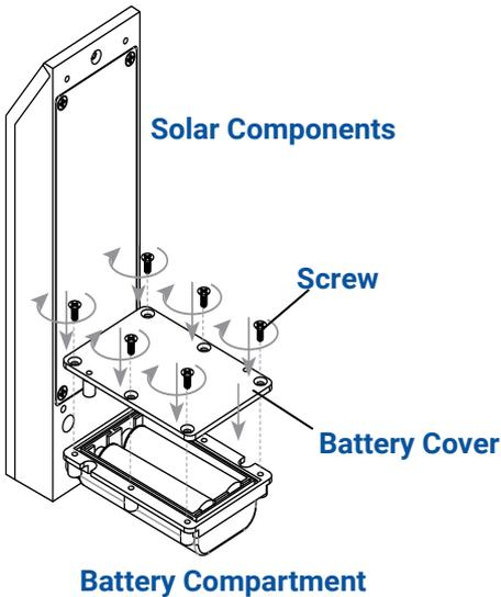
Place the battery cover back onto the battery compartment and secure with previously removed screws.
