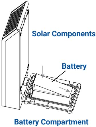
Insert two batteries into the battery compartment.
