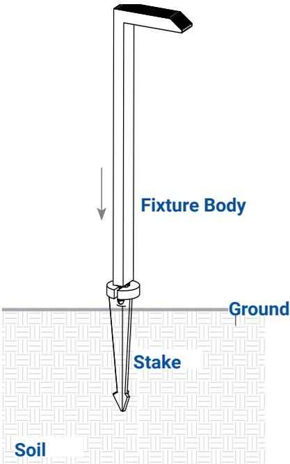
Insert the stake into the soil until flange of stake is flush to the ground.
