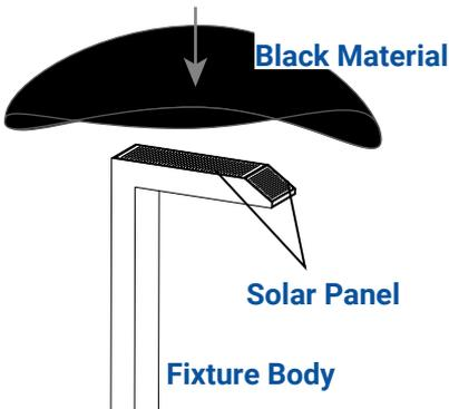
Cover solar panels completely by using black materials. The fixture will light up when the solar panel is covered and turn back off when it is uncovered.
