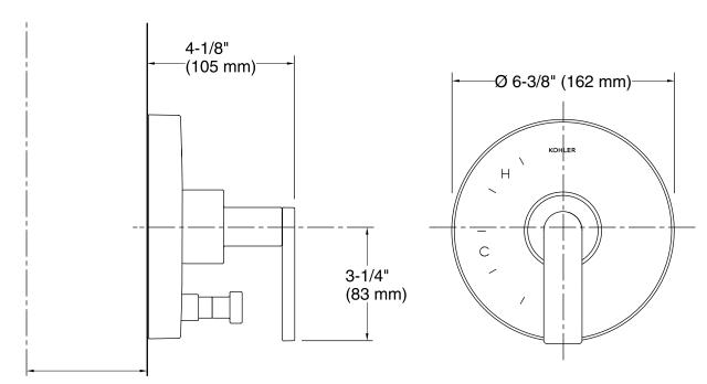
2-3/4" (70 mm) Thin Wall 3-1/2" (89 mm) Thick Wall If over 3-1/2" (89 mm) and up to 4-1/2" (114 mm), use Deep Roughing-in Kit
