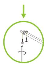
4. Hold the light strip with the clip and lock the screw.
