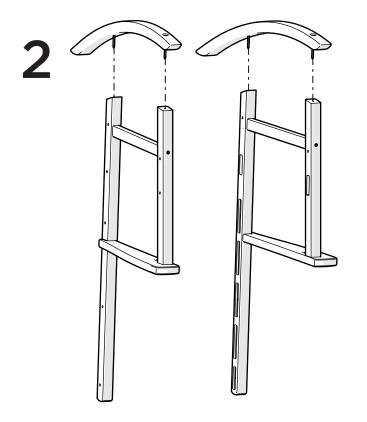
Partially thread each screw into pilot holes by hand before fully tightening.
