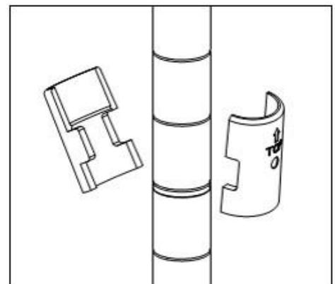
\* For safety and stability, the lowest SHELF (C) should be lower than the 3<sup>rd</sup> notch from the bottom.
