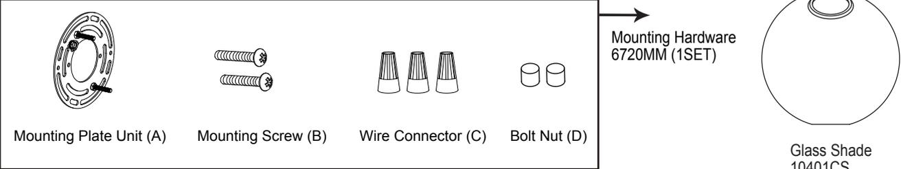
Mounting Plate Unit (A)    Mounting Screw (B)    Wire Connector (C)    Bolt Nut (D)
