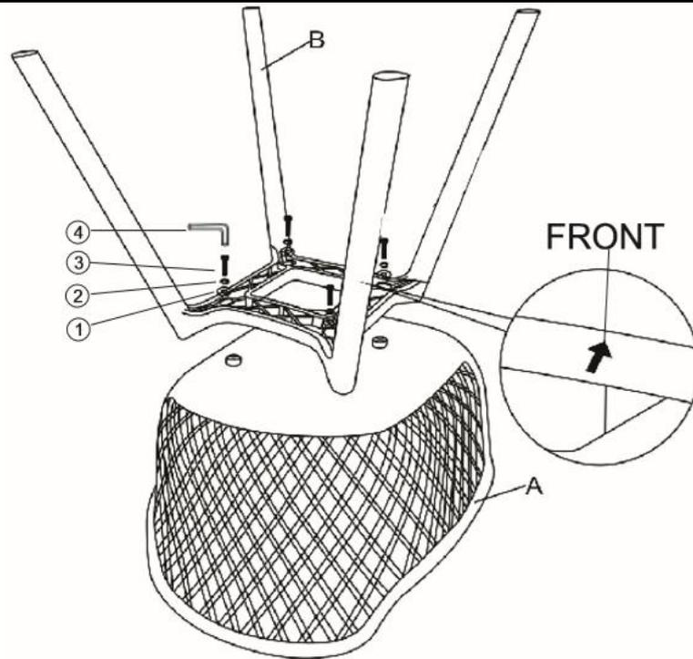
Place the Chair Seat (A) with its bottom side facing upwards onto a clean, soft surface to avoid any scratches or damage to the product.
