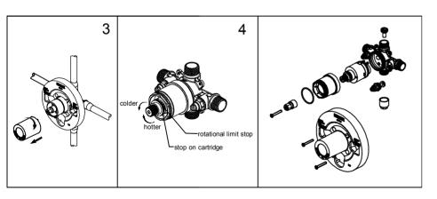
3. Before installing escutcheon, remove the plastic cap from plaster guard by twisting cap in a clockwise direction. Remove the screw from the inverter.
