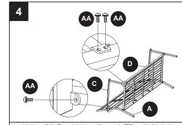
Hand tighten (AA). Do not tighten with wrench (BB), until all bolts have been installed.
