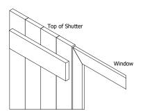
**2)** When Installing Shutters Smaller than 55", Drill (4)  $^{5}/_{16}$ " Holes into the Shutter ONLY, in the Locations Shown in Figure 1 to the Right.
