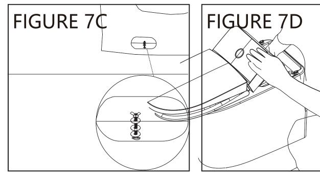
Caution: Do not move the toilet bowl around once the toilet bowl is in position. It can damage the wax ring seal and result in water leakage.
