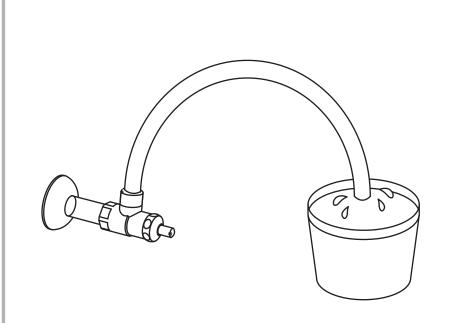
Open the angle valve for water supply. The measured water flow for 10 seconds should exceed 3L.
