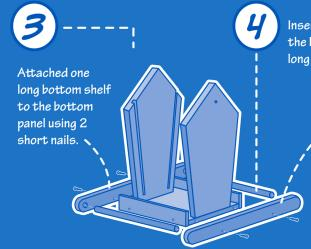
Insert the round rods into the holes on the attached long bottom shelf.
