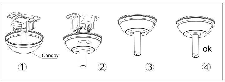
Raise canopy to hanging bracket, aligning loosened screws in hanging bracket with slotted holes in canopy. Twist canopy to lock. Re-insert screws and secured all screws with screwdriver.
