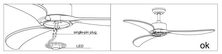
Unscrew a set screw. Attach the LED pan up to the bottom of the fan by inserting the other two set screw heads into key hole slots, rotate it to place, then secure the previous set screw by aligning screw hole and the hole at the bottom of the fan, tighten the rest two set screw to secure LED pan.
