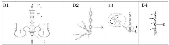
Step B1: Carefully thread post (M) onto the fixture (O), then thread the loop (L) onto the post (M).
