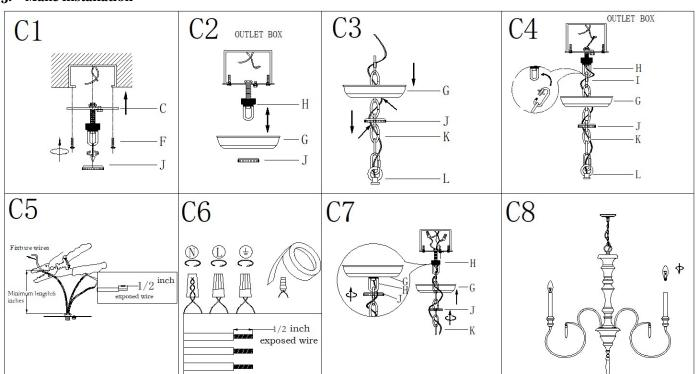
Step C1: .Attach single bar (C) to outlet box with mounting screw (F). The side of single bar marked "GND" must face out.
