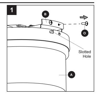
Slide the motor housing (A) over the motor (E), aligning the slotted holes in the motor housing (A) with the loosened motor housing screws (O) in the upper mounting bracket (B). Twist the motor housing (A) clockwise to lock. Then re-insert the two previously removed motor housing screws (O) and securely tighten all screws.
