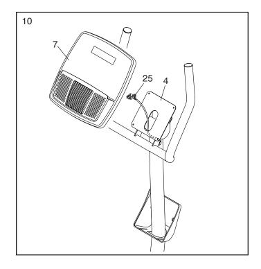
11. **Tip: Avoid pinching the Main Wire (25).** Attach the Console (7) to the Handlebar (4) with four M4 x 16mm Screws (2); **start all the Screws, and then tighten them.**
