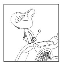
the seat post knob. Move the seat post upward or downward slightly to make sure that the seat post knob is engaged in one of the adjustment holes.
