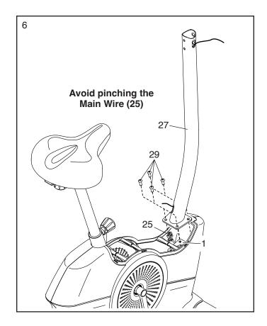
Locate the lower end of the wire tie (E) in the Upright (27). Tie the wire tie to the Main Wire (25). Then, pull the upper end of the wire tie until the Main Wire is routed through the Upright and out of the indicated hole (F).
