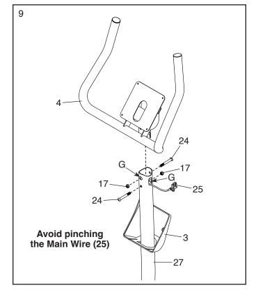
10. Untie and discard the wire tie on the Main Wire (25). Then, route the Main Wire upward through the Handlebar (4) as shown.
