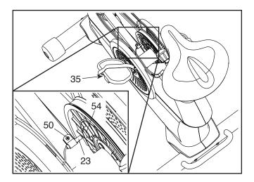
Next, rotate the Left Crank Arm (35) until a Magnet (54) is aligned with the Reed Switch (23). Slide the Reed Switch slightly toward or away from the Magnet. Then, retighten the M4 x 19mm Screw (50).
