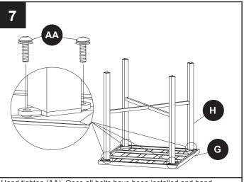
Hand tighten (AA). Once all bolts have been installed and hand tightened, go back and tighten firmly with wrench (BB).
