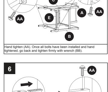
Hand tighten (AA). Do not tighten with wrench (BB), until all bolts have been installed.
