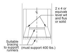
equivalent runners level with bottom of cutout and flush with sides of cutout or solid bottom floor.
