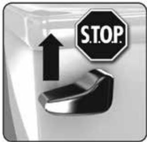
At the first sign of a clogged toilet, push handle upward as shown in the picture above.
