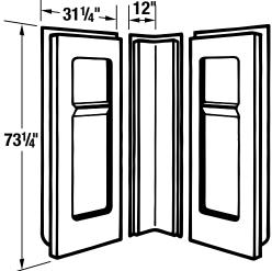
**General:** Furnish and install as shown on plans, 42" neo-angle shower, DURAWALL® Shower Walls Model 742C, as manufactured by E.L. Mustee & Sons, Inc. Shall be 3-piece, molded fiberglass wall with minimum thickness of 125 mils and mounts direct-to-studwalls. Includes center panel with molded-in shelves and two side panels with molded-in shelf. Self aligning panels use a tongue-and-groove connection. Shall meet ANSI Z 124-2011.2. Color: \_\_\_\_\_ (White)
