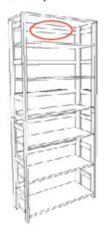
STEP 2a: Attach the Strap(C) to the highest cross brace that spans the back of your bookcase with 2 Small Screws (A).
