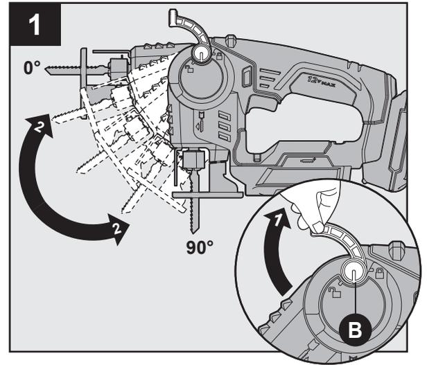
**!** **WARNING:** When adjusting the tool, only hold the foot plate (L) as shown below. **NEVER** hold the pivot head.
