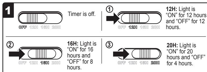
1 Slide the timer switch to 'OFF' before pressing any of the color push buttons (White, Blue, or Red). When the timer is off, turn the light on and off manually by pressing the color push buttons.
