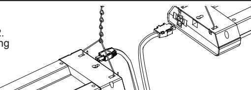
**NOTE:** The linking cord is designed to attach one way and only one way into the adjoining fixtures. If the plug cannot be fully inserted into the fixture, reverse the ends of the cord and try again.
