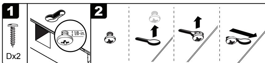
1 Adjust the screws (D), leaving 1/8-in. clearance between the mounting surface and the back of the screwhead.
