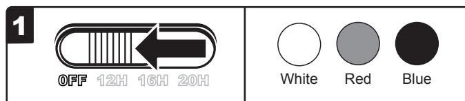
1 Slide timer switch to 'OFF' before pressing any of the color push buttons (White, Blue, or Red). When the timer is off, turn the light on and off manually by pressing the color push buttons.
