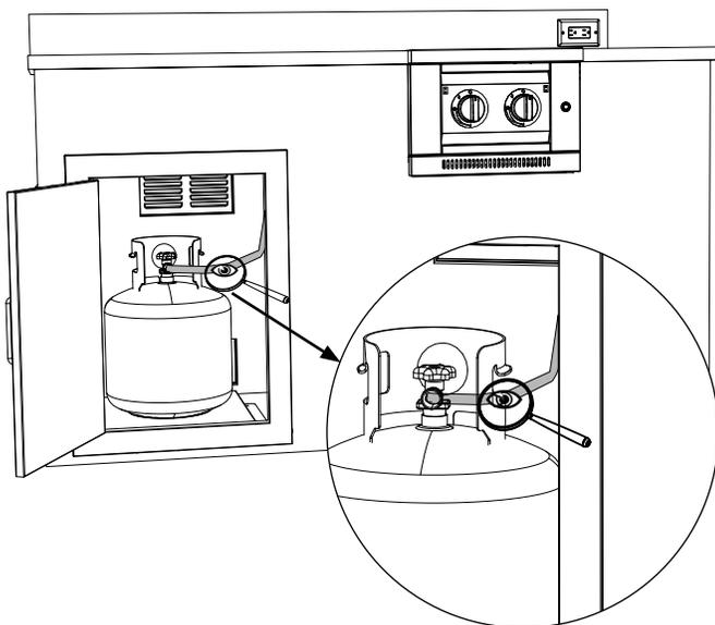
HOSE SHOULD HAVE A SMOOTH SNAKED PATH TO PREVENT KINKS AND PREMATURE FAILURE. PLEASE EXAMINE HOSE AND FITTINGS FOR CRACKS, TEARS, OR WEAR MARKS FROM RUBBING ETC.
