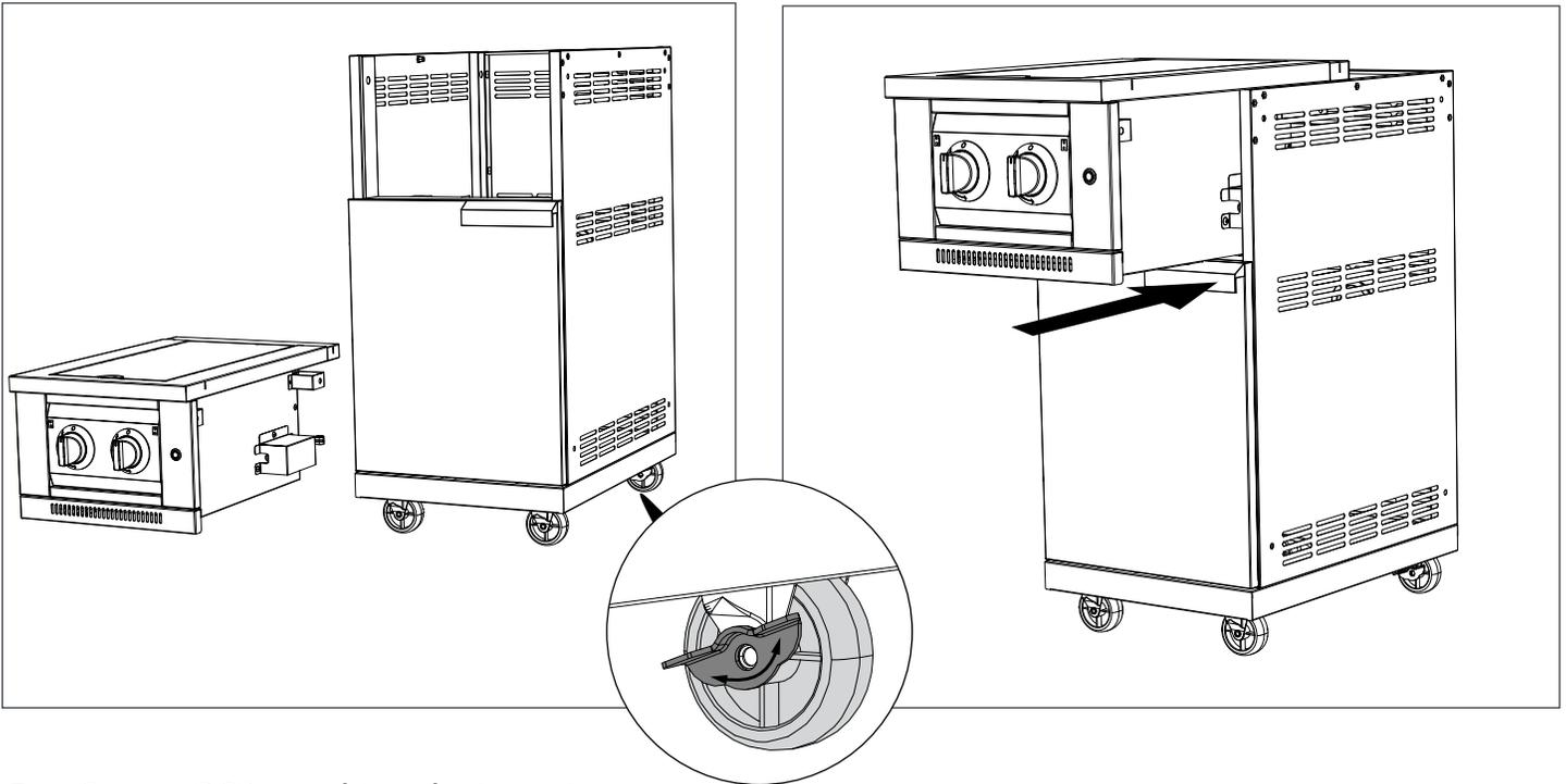
**3** Secure DSB to cabinet by inserting two M6x12mm from the bottom. Flat head screws are provided with the DSB.
