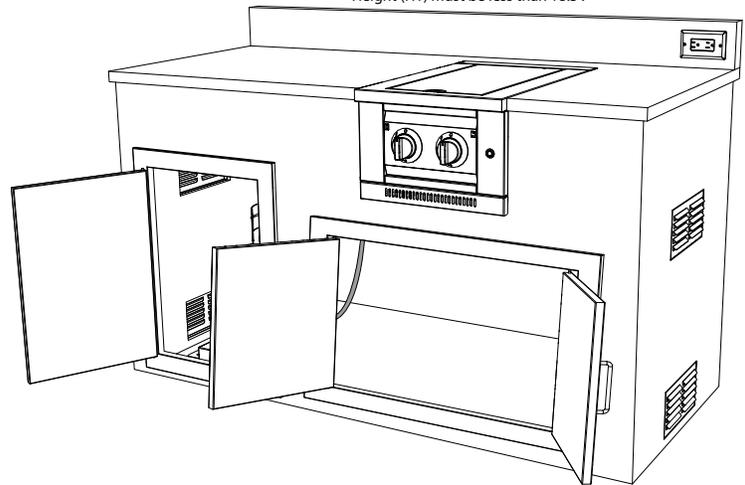
propane tank must be secured to the built-in cabinet inside the cylinder enclosure.
