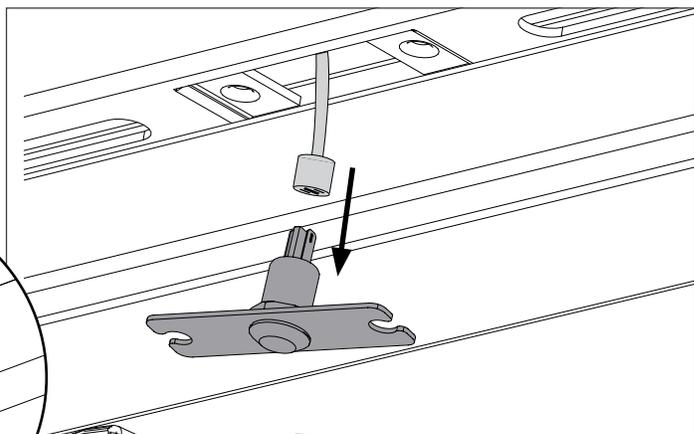
**3** Loosen the lock nut and replace the LED Bulb.
