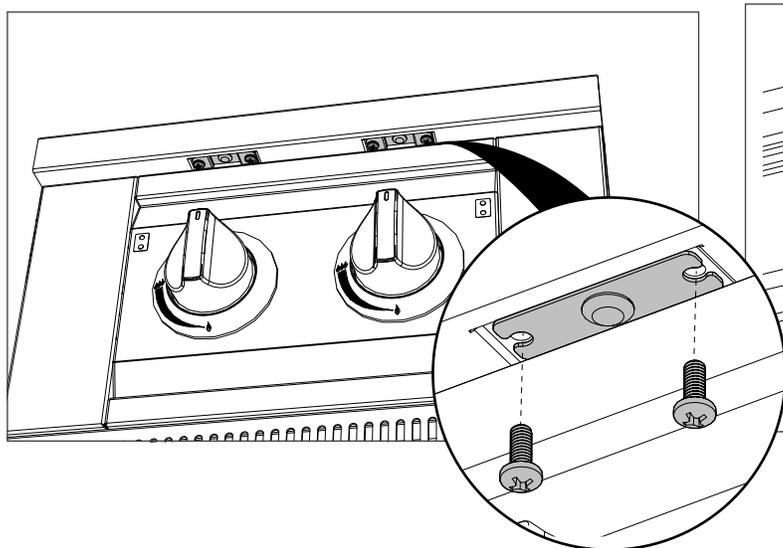
**2** Remove the LED light assembly and disconnect it from the power connector.
