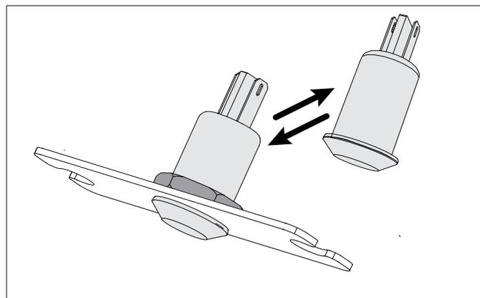
**4** Connect the LED light assembly to the power connector and secure it to the grill with the two screws using Phillips head screw driver.
