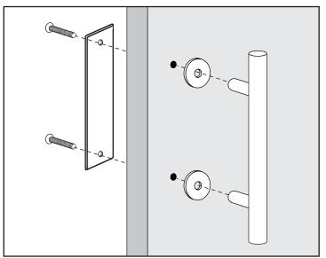
Insert the (2) M8x60mm screws through the square flush plate and install through the door and secure the handle on the exterior.
