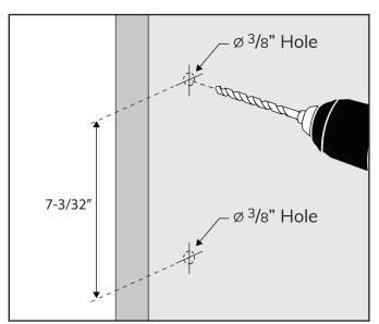
Mark the mounting holes 7" apart center on center and drill (2) <sup>3</sup>/8" diameter holes as shown in the illustration below.
