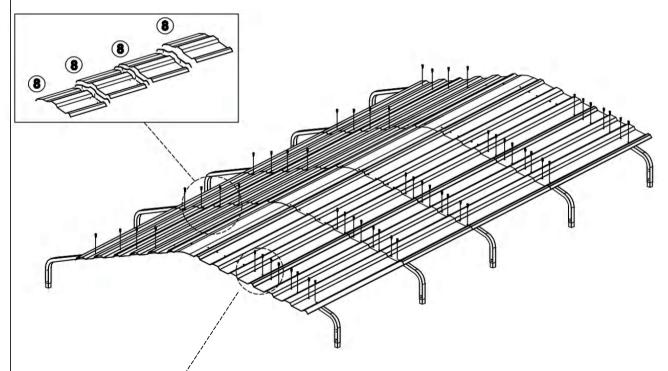
The color steel tiles should be layed and pressed one piece by one piece tightly to prevent rain.
