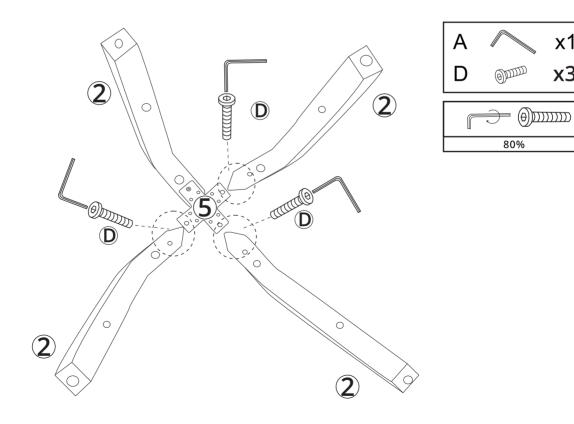
**3** First install the footrest ③ and tighten its screws to 80%. Then tighten all screws on footrest ③ to 100%. Finally tighten all screws on connecting frame ⑤ to 100%.
