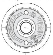
CAUTION: RISK OF FIRE - USE 15 WATT OR SMALLER, 120 VOLT, TYPE C LAMP ATTENTION: RISQUE D'INCENDIE -UTILISER EXCLUSIVEMENT DES LAMPES DE CLASSE C DE 15 WATTS
