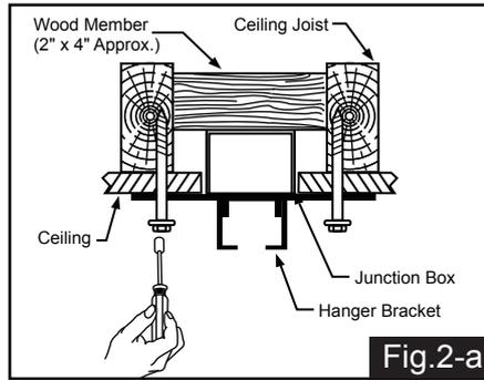
Tighten the hanger bracket to the outlet box with two mounting screws. **(Make sure the outlet box is securely installed so that it will be able to support at least the fan weight.)** Attach the safety cable hook to the ceiling with the drywall screw and washer, and make sure the safety cable hook is covered by the fan canopy. **WARNING: MOUNT ONLY TO AN OUTLET BOX MARKED "ACCEPTABLE FOR FAN SUPPORT"!**
