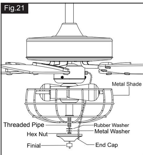
Install the metal shade, rubber washer and metal washer upward through the threaded pipe and secure with hex nut. Then attach the end cap to the metal shade and secure it with finial. Take care to align the holes on the metal shade and the end cap, so that the pull chains pass through and move freely.
