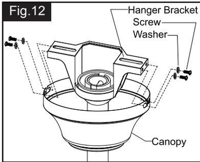
There are four hanger bracket screws and lock washers. Remove two screws and lock washers from the hanger bracket (one from each side) and loosen the other two remaining screws. Align the "L shaped" slots of the canopy with the two remaining screws on the hanger bracket and push the canopy upwards to engage the slots and turn clockwise to lock in place. Tighten the screws and install the other two hanger bracket screws and lock washers into the remaining holes of the canopy and tighten.
