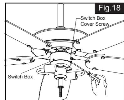
Secure the switch box cover onto switch box with the switch box cover screws.
