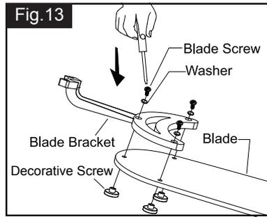
Tighten blades to blade brackets by using blade screws, washers and decorative screw.
