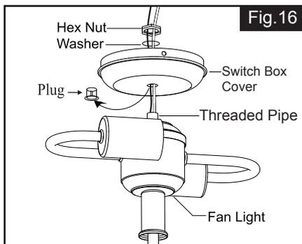
Remove the plug from the switch box cover. Remove the nut and lock washer from fan light. Attach the fan light to the switch box by threading the fan light wires (black and white) and remove threaded pipe through the hole of switch box and then secure them onto the switch box with hex nut & washer. Be sure it is tight enough to prevent light kit from vibrating loose.
