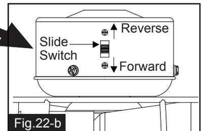
The slide switch on switch box sets direction of fan rotation. Select the desired direction of fan rotation. Push the slide switch down for "Forward" and up for "Reverse".
