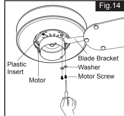
Remove the motor screws and washers from the fan motor assembly. Secure blade brackets to the motor with washers and motor screws.
