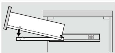
Pull forward until the peg engages with the fixing holes in the drawer base.
