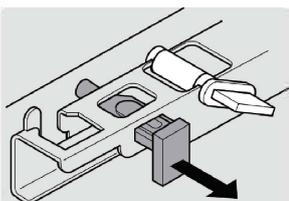
Open the lock by pushing the peg out of the hole.
