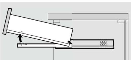
Pull the peg out of the fixing holes in the drawer base.
