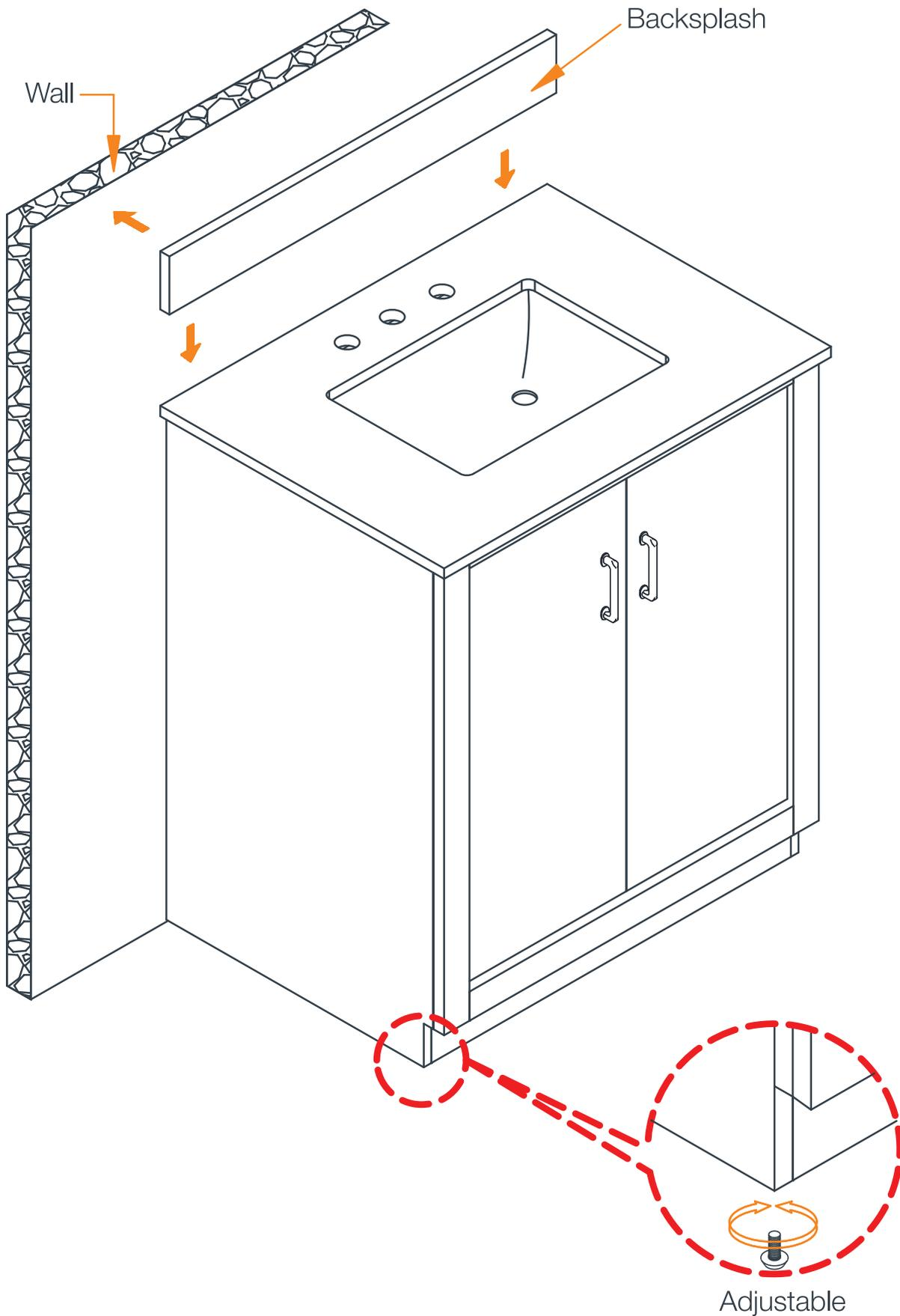
For application of backsplash (B) to drywall: Make sure the wall is smooth and flat. Clean the wall and the back of the backsplash (B) with damp cloth to remove any grease or debris. Apply thin-set adhesive, and then set the backsplash (B).
