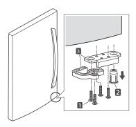
Reinstall the hinge pin brackets 1, screws 2 and hinge pin insert 3 on the bottom left side of the door.
