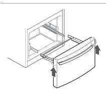
6 Holding one rail with each hand, push the rails in simultaneously.
