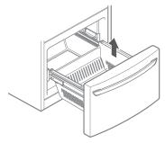
3 Remove the screws at the ends of both rails.
