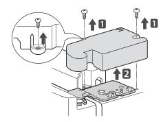
2 Using a13/32 in. or 10 mm socket wrench, remove the three bolts and lift off the top hinge. Set parts aside.
