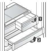
To install, slightly tilt up the front, insert the drawer into the frame and push it back into
