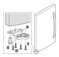
6 Use a ¼ in (6.35 mm) hex socket wrench to loosen the hinge pin 1 and remove. Remove the two bolts 2, the screw 3 and the hinge 4.
