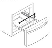
Grip both sides of the drawer and pull it up to remove it from the rails.
