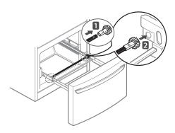
4 Lower the door into final position and tighten the screws located on both sides.
