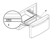
With the drawer pulled out to full extension, insert the lower basket in the rail assembly.
