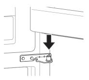
2 Line up the top hinge with the holes in the top of the refrigerator. Use the three bolts to replace the hinge. Tighten the bolts.
