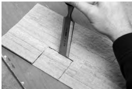
Cutting the inside edge with chisel
