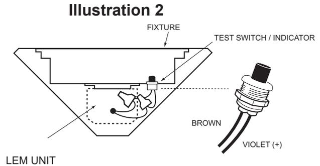
NOTE: Position the **Test Switch/Indicator** so that it can be seen after installation.
