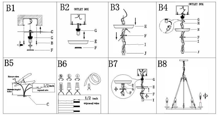
Step B1: .Attach the single bar (E) to outlet box with mounting screws (B). The side of single bar marked "GND" must face out Step B2: Raise the canopy (G) through screw collar loop (I) and screw the collar loop (I) to a proper position by measuring.
