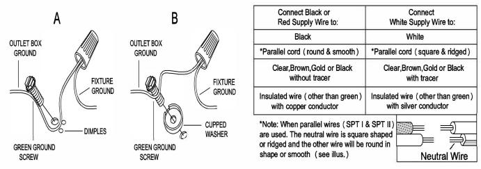
Twist plastic wire connector until wires are tightly joined together, wrap each connector with approved electrical tape. Be sure that no wire strands are exposed and then carefully tuck all wires into the outlet box. Step B7: Raise canopy (E) to ceiling and secure canopy (E) in place by tightening threaded ring (F) onto collar loop (G). Step B8: Install the bulb (not included) (Please do not exceed the maximum capacity recommended on the socket.)
