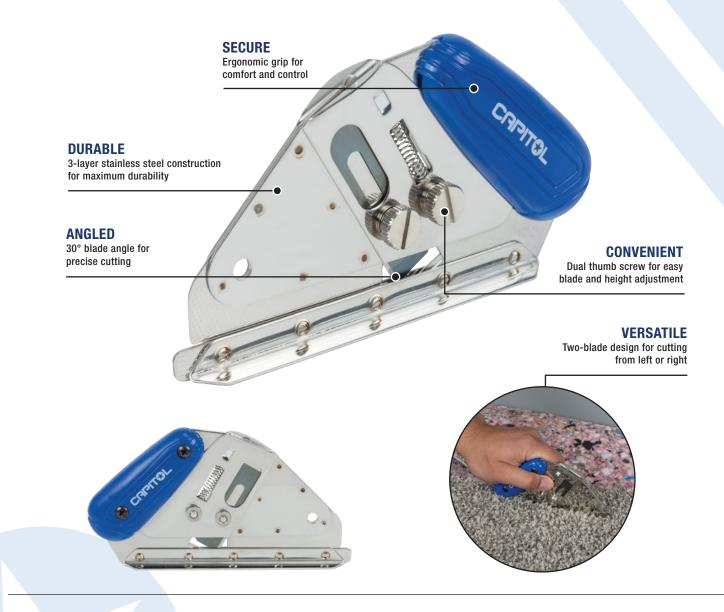
Capitol<sup>®</sup> Professional Loop Pile Carpet Cutter is designed to cut all thickness of loop pile carpet, and trims carpet with ease and precision. The two-blade design accommodates left or right-handed cutting, while ergonomic grip improves comfort and control.
