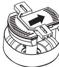
1. Carefully push the canopy to the bottom of the mounting bracket, make two sliding holes aligned to the two prominent screws on the mounting bracket, and then turn clockwise until tight.
