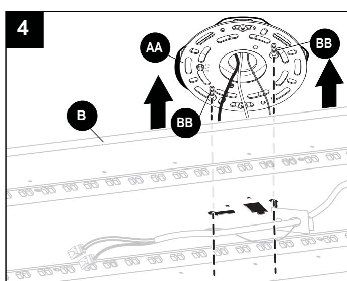
5. ① Insert the box screw (BB) heads into the large round ends of the keyhole slots. ② Slide the fixture until the screw (BB) heads are fully captured by the narrow portion of the keyhole slots. Pivot the fixture to align with chosen wall, while keeping both box screws (BB) engaged in the narrow slot.
