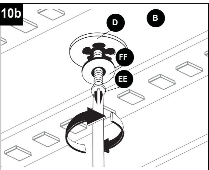
10b. WOOD: If the ReadyAnchor™ (D) does not fully seat due to interference from a wooden stud, break off the ReadyAnchor™ (D) from its plastic base. Drill a 3/32 in pilot hole in the center of where the ReadyAnchor™ (D) was. Place one of the included washers (FF) over the wood screw (EE) and securely fasten it directly to the stud. DO NOT OVERTIGHTEN.
