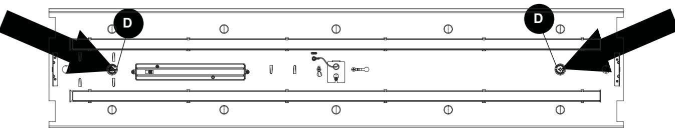
10a. DRYWALL: For added support on the outer ends, use a handheld Phillips head screwdriver to drive the pre-installed ReadyAnchor™ (D). As the ReadyAnchor™ (D) turns, it will break free from its plastic base. Continue turning to puncture into the drywall and tighten until the ReadyAnchor™ (D) bottoms out. Do not OVERTIGHTEN.
