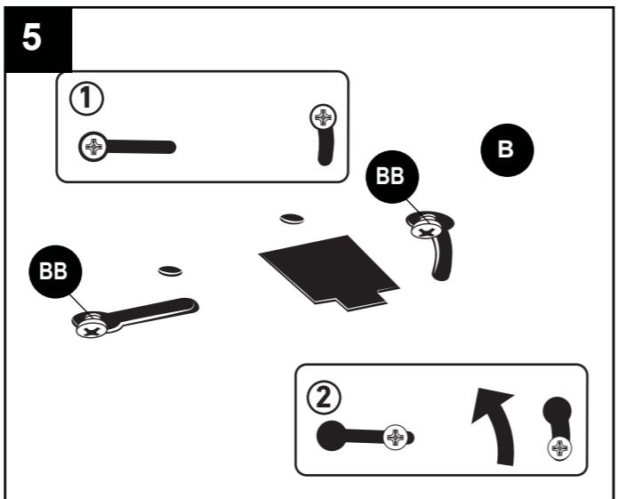
6. Once both screws (BB) are fully engaged in the narrow channels of the slot, maneuver the fixture into its desired position and tighten the screws (BB). DO NOT OVERTIGHTEN.
