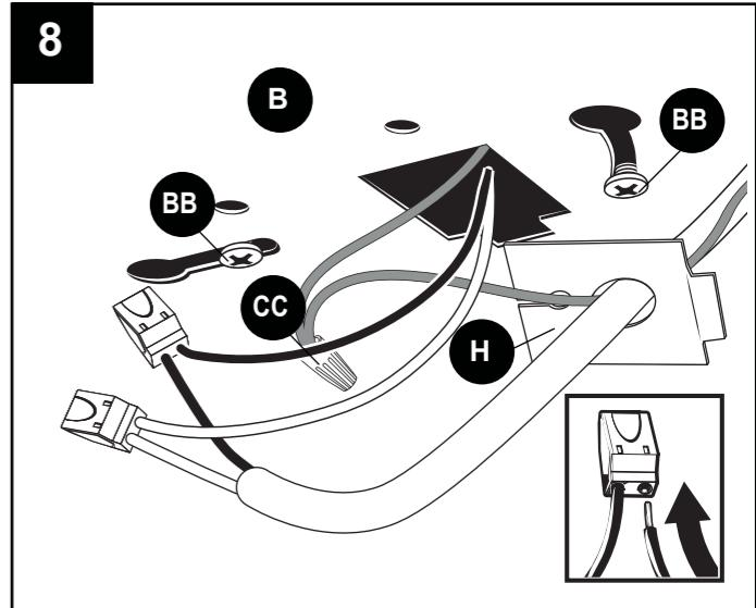
9. Push all the connectors and excess wire into the electrical box and reattach the wire cover (H).
