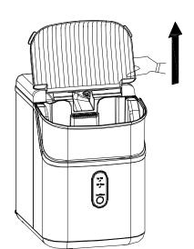
**Tips**: remove the top back cover by pulling up the front transparent cover gently.
