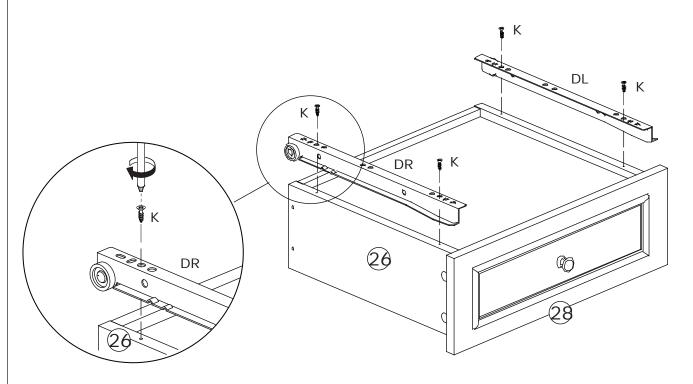
Fix runner(DL) and (DR) to plate #25 and #26 with screw(K) as shown.
