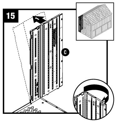
Tip left front (C) outward slightly and bend corner hinge.
