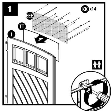
Stand left door (I) vertically. In this order, layer into door channel the window gasket (TT), and door window (EEE). Through the back of door, secure layers with fourteen screws (KK). Start with four corner screws and finish with remaining screws. **DO NOT** over tighten screws.
