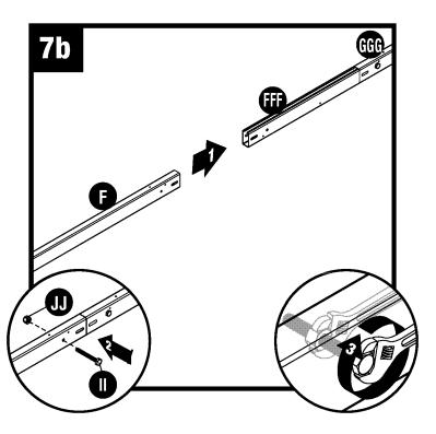
Place ridge beam (F) onto the ridge beam joiner (FFF). Secure with hex bolt (II) and nut (JJ).
