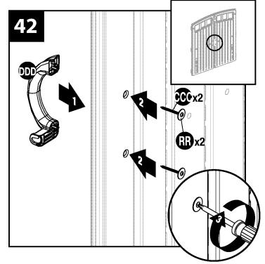
Attach door handle (DDD) to left door with two screws (CCC) and two washers (RR). Repeat for right door.
