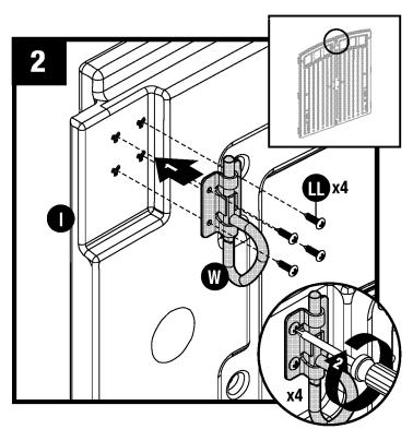
At top interior side of left door (I), attach D-ring slide bolt (W) with four screws (LL) through provided holes.
