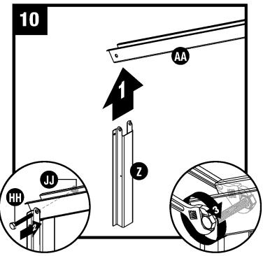
Place side adaptor bracket (Z) at end of left truss leg (AA). Secure adaptor bracket with one 2" hex head cap screw (HH) and one nut (JJ).
