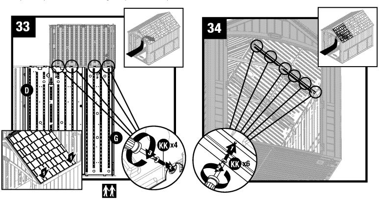
Pull down each lower corner of roof from outside. From inside shed, attach tabs on side panel (D) and right front (G) corner to roof panel with four screws (KK).
