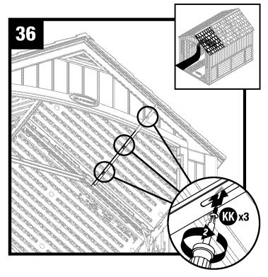
Secure roof support (WW) to roof using three screws (KK).
