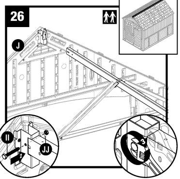
Slide ridge beam into front roof ridge beam bracket. Secure with 1 1/2" hex head cap screw (II) and nut (JJ).
