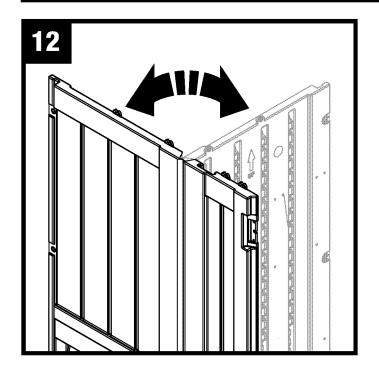
**Critical:** When installing corners, flex corner hinges back and forth several times. This will help provide a square corner and ensure proper fit of remaining panels.
