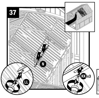
Raise roof support (N) into position against roof. Secure roof support (N) to truss leg with one screw (LL) on each side. Secure roof support (N) to roof using three screws (KK). Repeat steps 33-37 to secure remaining roof panels.
