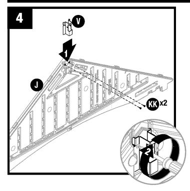
Slide roof ridge beam bracket (V) under tabs on inside peak of front header (J) and secure with two screws (KK). **DO NOT** over tighten screws.
