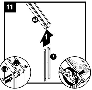
Place side adaptor bracket (Z) at end of right truss leg (AA). Secure adaptor bracket with one 2" hex head cap screw (HH) and one nut (JJ). **Repeat steps 8-11 for second truss.**
