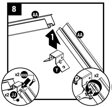
Attach truss bracket (Y) to end of one truss leg (AA) with 1" hex head cap screw (HHH) and nut (JJ).
