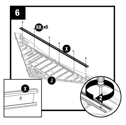
Lay header (J) on ground with lettering side facing up. Place one header beam (X) into pocket on inside of front header (J). Attach with six screws (KK). **DO NOT** over tighten screws.
