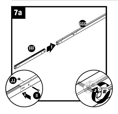
Place ridge beam joiner (FFF) into the ridge beam (GGG). Secure with hex bolt (II) and nut (LL).
