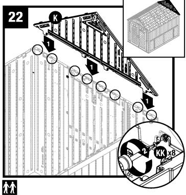
Place rear header (K) over back walls and fit four protruding support legs into pockets molded in back walls. Secure rear header using eight screws (KK).
