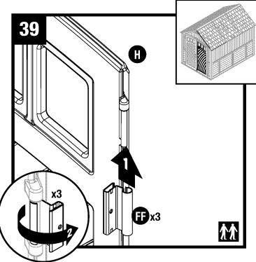
Stand right door (H) upright with three hinge mounts facing right. Slide one metal hinge plate (FF) up onto each hinge mount. Rotate hinge plates to outside of door. Snap metal hinge plate into place by pushing
