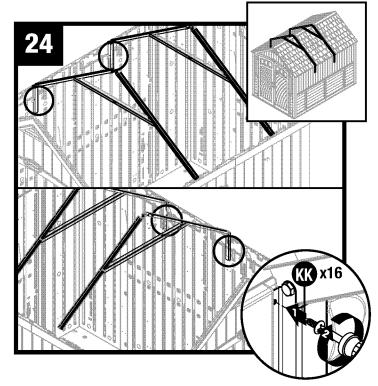
Secure with four screws (KK) in each side adaptor bracket.
