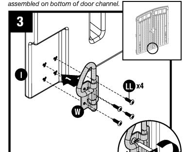
At bottom interior side of left door (I), attach D-ring slide bolt (W) with four screws (LL) through provided holes.
