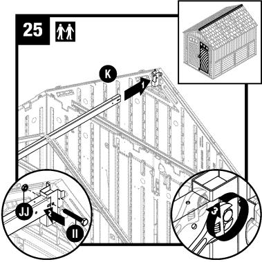
Raise ridge beam up and into rear header (K) Secure with 1 1/2" hex head cap screw (II) and nut (JJ).
