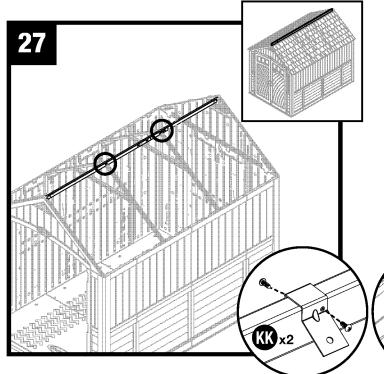
Attach the roof truss assembly to the ridge beam with two screws (KK).
