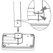
Please note that there are two different ways you can attach the pole to the base, depending on how you will be mounting it outdoors. If you will be fastening the sensor directly to a railing, use the option that positions the stand perpendicular to the sensor pole. If you will be fastening it to a pole, use the slot that positions the base parallel to the sensor pole.
