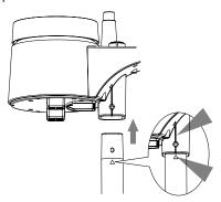
2. Insert the nut into the hexagonal hole by the sensor and hold it in place, then insert the screw through the other side. Use a screwdriver to tighten the screw. Do not insert the screw first, or the nut may not line up correctly with the designated hole.
