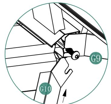
Tighten the screw (X3) halfwy , then install the fix beams (G9 and G10) , finally tighten the (X3)
