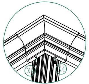
step20 1-Slide 5 Hooks(Q) into long sides beams(W/W1).
