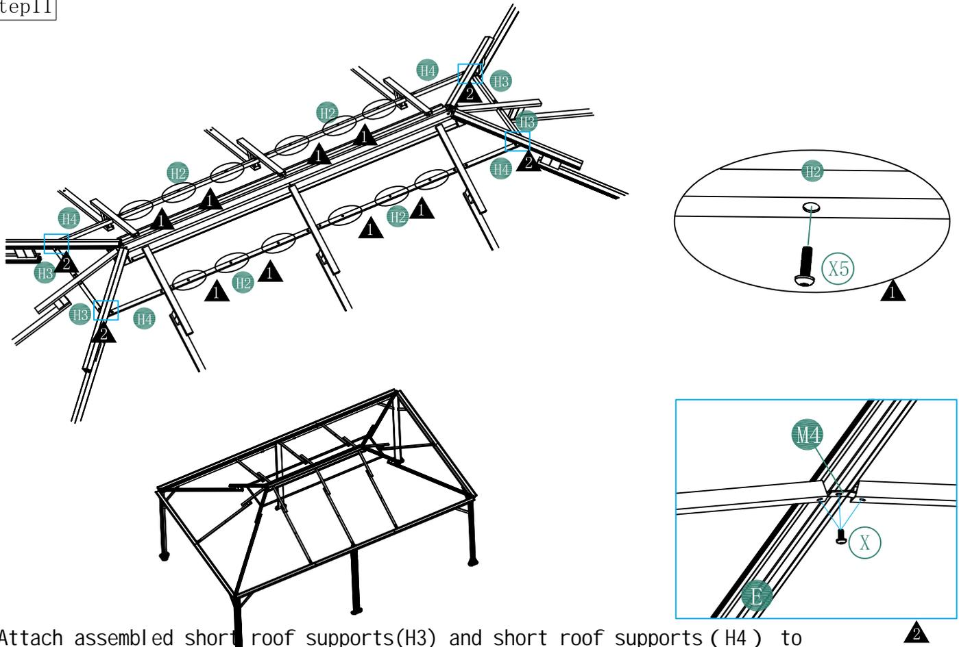
Attach assembled short roof supports(H3) and short roof supports (H4) to connectors (M4) , fix by using Bolt (X) ; then long roof supports (E) to connectors (M4) , fix by using Bolt (X)
