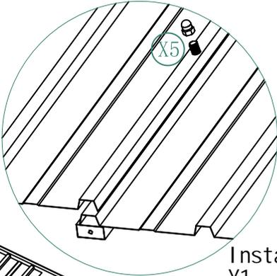
Install the Roof Plates (N1, N2, N3, N4, N5, N6, Y1, Y2, Y3, Y4, Y5) on the Long Sides of the Gazebo. fix by using bolt (X7, X5, X2)
