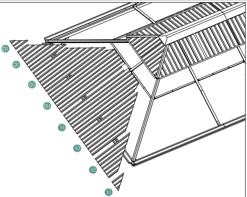
Install the Roof Plates (O1, O2, O3, O4, V1, V2, V3, V4) on the Long Sides of the Gazebo. fix by using bolt (X7, X5, X2)
