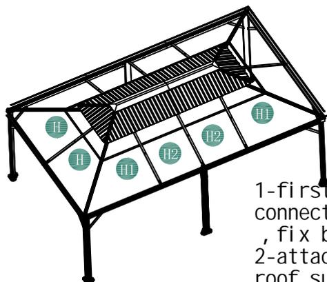
1-first attach the 2 short roof supports(H2) to connectors(M3), and short roof supports (D) to connectors (M3) , fix by using Bolt (X/X5)
