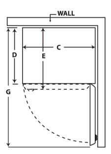
Allow sufficient clearance on hinge side of refrigerator when installing next to a wall where handle may make contact.
