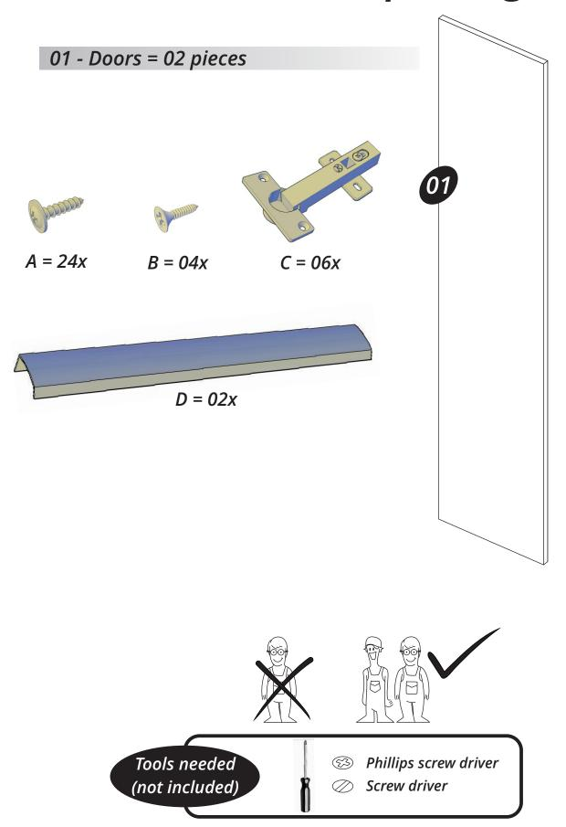
Attention to the position of the Handle (D) on the part (01). One up and one down.
